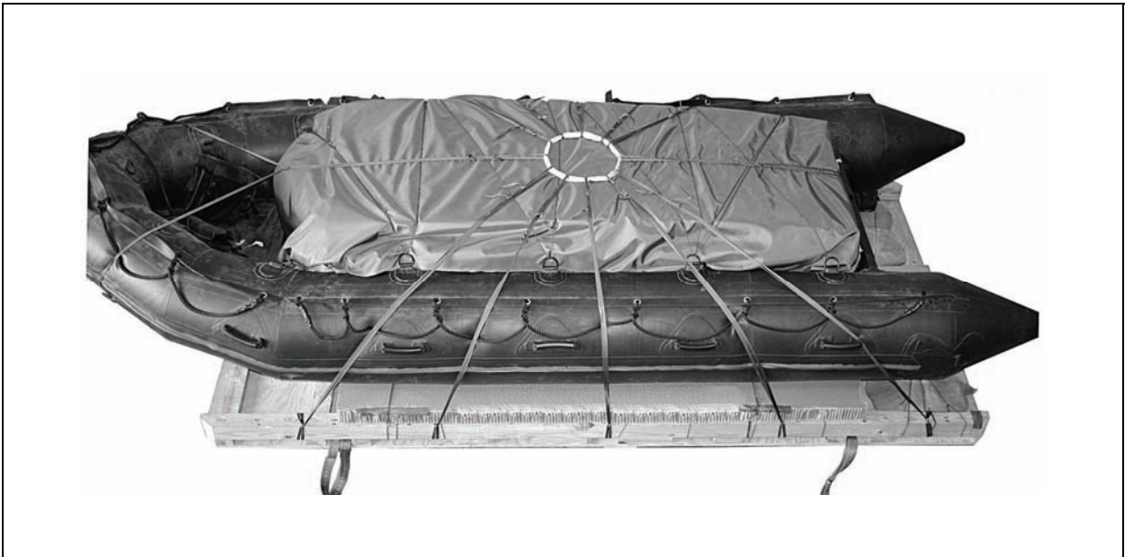
Figure 2-31. Load Covered, Tied in Place and Boat Lashed to Platform
